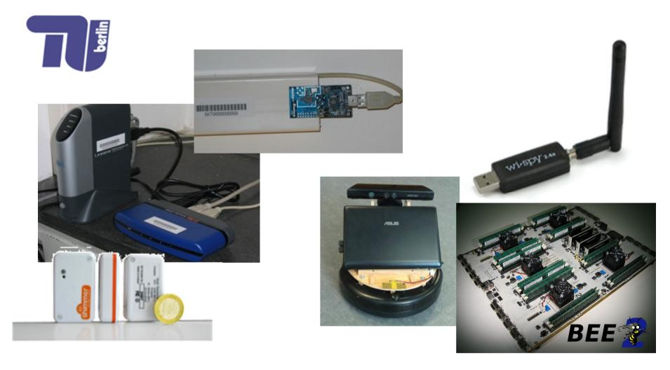
204 +16 wireless sensor nodes (Tmote Sky/EyesIFXv2/Shimmer2) cognitive components: Wi-Spy, BEE 2 FPGA platform
