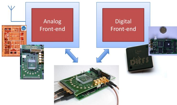
Advanced spectrum sensing Combination of analog & digital FE in compact device
