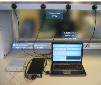
Transceiver API for SDR architecture (compliant to WINNF)
