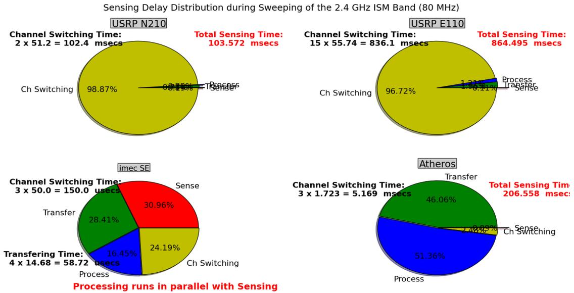
Figure 7: Sensing Delay Distribution during Sweeping of the 2.4 GHz ISM Band
