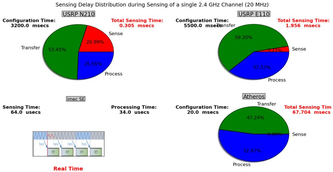
Figure 4: Sensing Delay Distribution during Sensing of a single 2.4 GHz Channel
