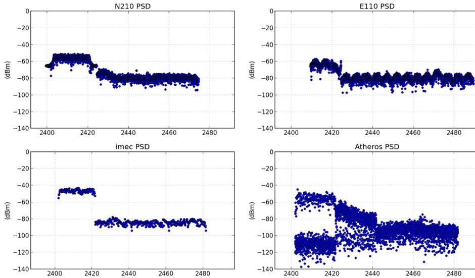
Figure 5: PSD Evaluation during Sweeping of the 2.4 GHz ISM Band
