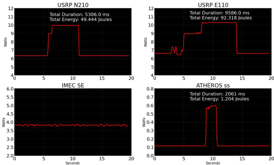
Figure 6: Energy Consumption during Sweeping of the 2.4 GHz ISM Band
