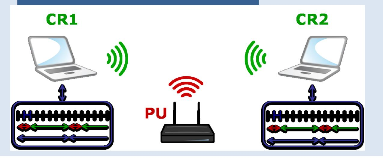
The Primary User (PU) floods its channel(s) to simulate the transmission activity in the licensed spectrum.
